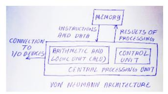
Computer architecture in based on Von Neumann Architecture.
